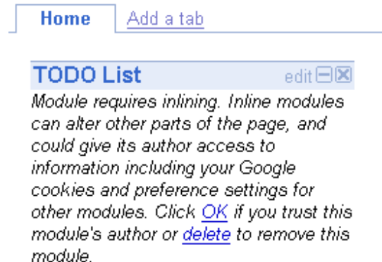
Figure 1: Example warning message from Google personalized homepage. This third-party “todo” list gadget requires inlining so that it can request additional height from its parent as more items are added to the list. Unfortunately, inlining also allows the gadget author to access the user’s Google account.
